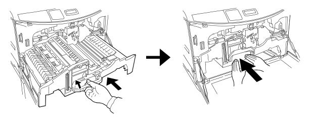
7. Turn the lock lever clockwise as shown in the figure to securely lock the feed unit.
